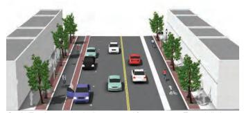
**Cycle Tracks** are physically separated from motor traffic and distinct from the sidewalk, providing a higher level of comfort and attracting a larger user base.
