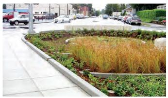
**Bioswales** remove silt and contaminates from surface water runoff and are commonly implemented near parking lots where vehicle pollution is aggregated.
