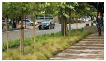
Pervious sidewalks not only provide the surface water to infiltrate, but also can enhance the visual aesthetics of the space.
